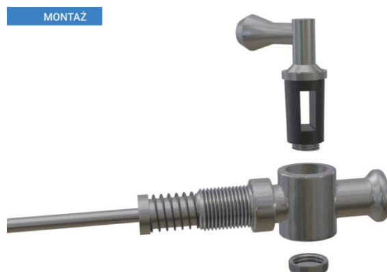
Figure 4. 3D animation 'Disassembly and assembly of medical equipment', Veress needle assembly
