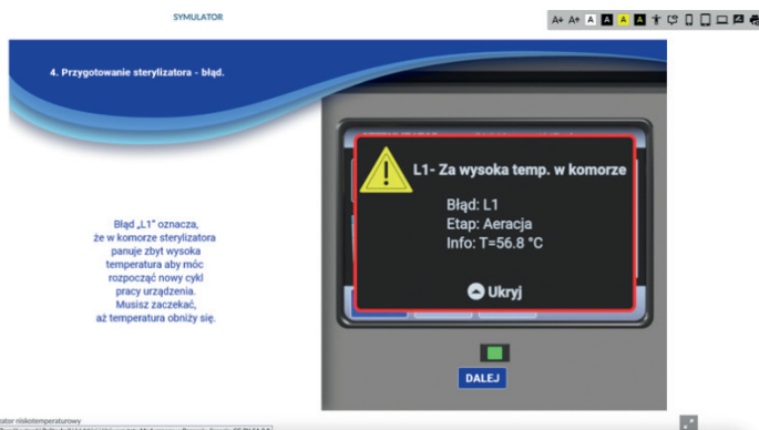
Figure 2. Low temperature – gas sterilizer simulator, error during the preparation of the device for operation
