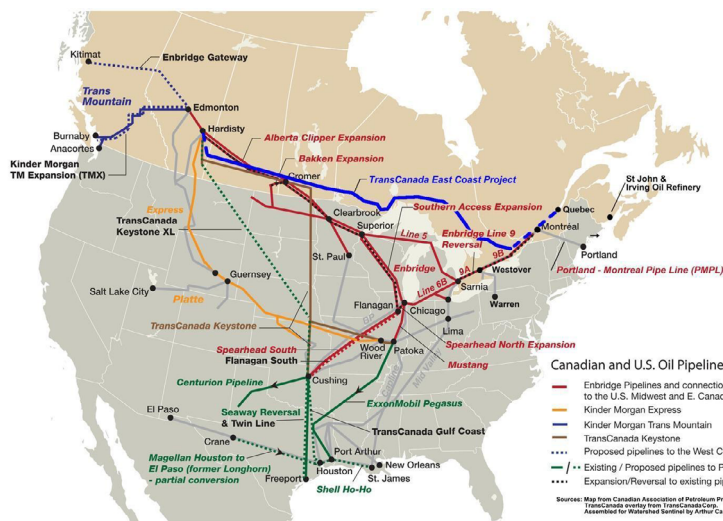
Fig. 1: Oil Pipelines from Canada's Tar Sands, Actual and Proposed, and Continental Oil Pipeline Infrastructure 2014. Source: Nelson, Joyce, "Line 9 - Shipping Tar Sands Crude East", November 7, 2012. By permission of Watershed Sentinel ( https://watershedsentinel.ca/articles/line-9-shipping-tar-sands-crude-east/ ).
