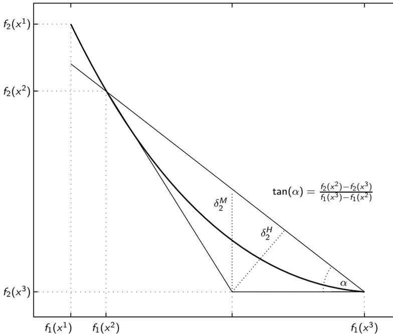
Figure 3. Illustration of error measures considered in Remark 1
